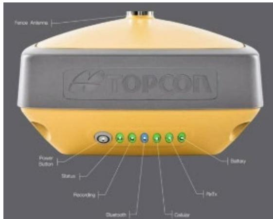
Hit « Start Occ » to start logging. Once duration is increasing. Check the third LED blink every second.
